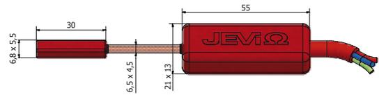
Twin conductor silicone cable with D terminal
