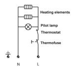
The overheating fuse is reconnected by pressing the button below the red nut on the connection box - after cooling down the drum heater. Any repairs must be made by an authorised electrician.
