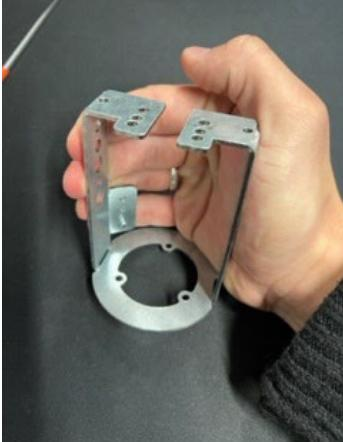
A photograph showing the same hand holding the bracket with the central vertical arm now fully compressed and inserted into the hole of the circular mounting plate. |
