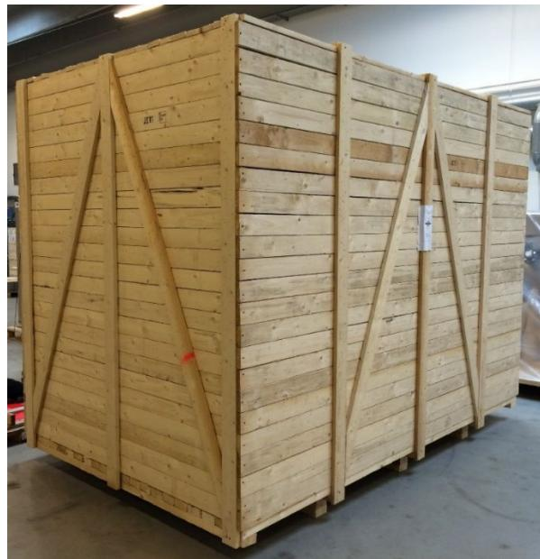
The packaging provides both mechanical and environmental protection. The Process heater is intended for service in an outdoor environment. However, to avoid any risk of harmful metallic dust during storage it is protected with enveloping plastic foil. All openings such as cable entry holes are adequately sealed.
