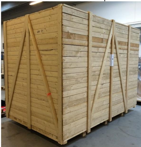
The packaging provides both mechanical and environmental protection. The Process heater is intended for service in an outdoor environment. However, to avoid any risk of harmful metallic dust during storage it is protected with enveloping plastic foil.
